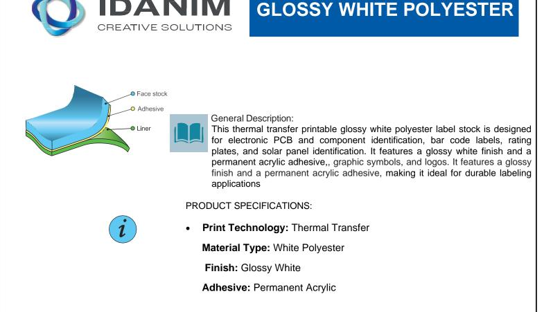
APPLICATIONS: This label stock is suitable for various applications including electronic PCB identification, bar code labeling, rating plates, and solar panel identification where high durability and clarity are required. **PHYSICAL PROPERTIES:**
