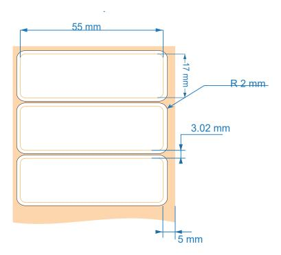
IDANIM PN :ILBDWPP55X17-1 CUST PN: 9220122 Importance of the CUSTOMER APPROVAL: Packaging MATERIAL : DURABLE POL DRAWING NR. : scrolling direction NAME: WINDING: OUT INNER CORE: 1 SIGNATURE: X IMPORTANT Knife number: 5434 TOLERANCE: ± 0,5 mm STAMP: SCALE: NOT IMPORTANT COLORS : WHITE 5 ♠♦ ↓ Format: **IDANIM** CUTTING LINE **DATE** :1.8.24 REVISION: 01 Idanim creative solutions: Moshe Hess St 7, Lod, Israel, Tel: 08-6225629 Fax: 08-6225629 e- mail: sales@idanimltd.com
